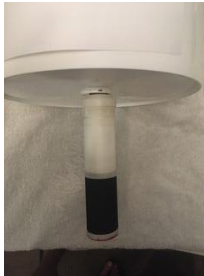
Photo showing the HI filter element hanging down from the bottom of the upper container
