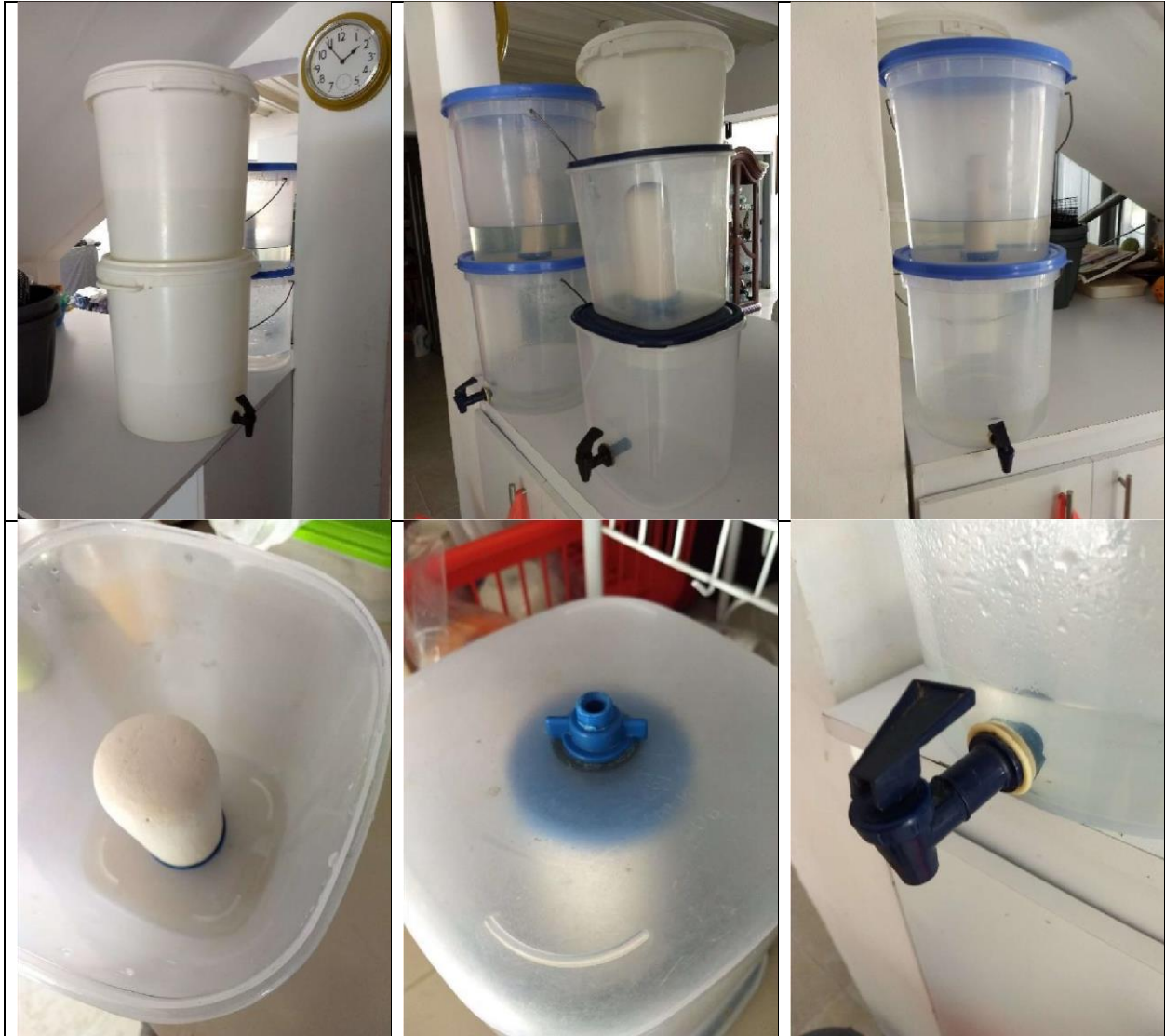
Photos of water filters made using JMCC GF Ceramic Water Filter Elements
